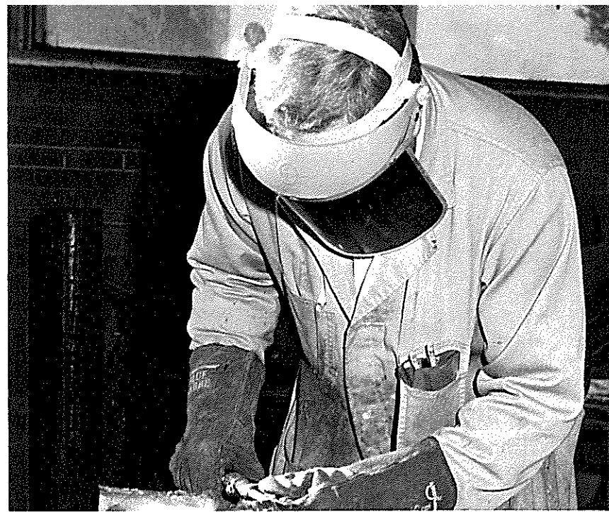
Ronny Stooksberry cuts some pipe demonstrating the use of a cutting torch in his Industrial Arts class.
