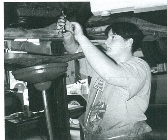
Cody Stephens changes the oil in a truck as part of a fund-raiser for the V.I.C.A. Club.
